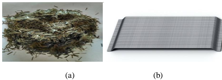
Figure 1: (a) Chopped basalt fibers and (b) Typical Hooked End Steel fibres
